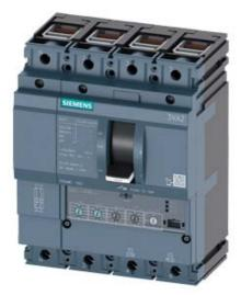
CIRCUIT BREAKER 3VA2 IEC FRAME 160 BREAKING CAPACITY CLASS C ICU=110KA @ 415 V 4POLE, LINE PROTECTION ETU350, LSI, IN=160A OVERLOAD PROTECTION IR=64A ...160A SHORT CIRCUIT PROTECTION ISD=1,5... 10 X IR, II=10 X IN **NEUTRAL PROTECTION** ADJUSTABLE(OFF,50%,100%) CABLE CONNECTION
