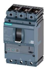
CIRCUIT BREAKER 3VA2 IEC FRAME 160 BREAKING CAPACITY CLASS M ICU=55KA @ 415 V 3POLE, LINE PROTECTION ETU320, LI, IN=25A OVERLOAD PROTECTION IR=10A ...25A SHORT CIRCUIT PROTECTION II=12 X IN BUSBAR CONNECTION
