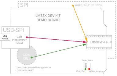
Power via • USB • Coin Cell • Arduino
