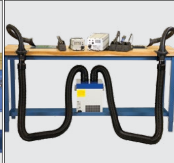
Arm-Evac 200 or 250 (Arm-Evac 200 shown. See pages 4-5 for specifications.) Two 50mm 24" Long ESD Flex Arm: P/N 8882-0415-P1 Two 50mm Bench Mounting Kit: P/N 8886-0553-P1
