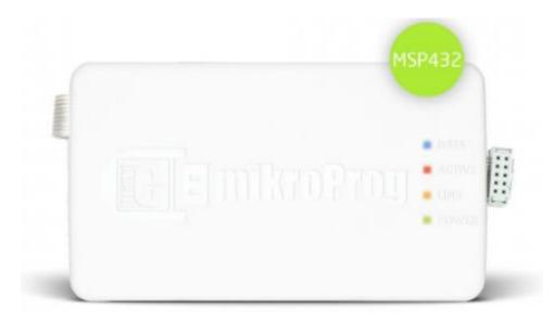
mikroProg<sup>™</sup> for MSP432 is a fast and reliable USB programmer and hardware debugger. This mikroProg supports the SimpleLink<sup>™</sup> MSP432<sup>™</sup> microcontroller family from Texas Instruments.
