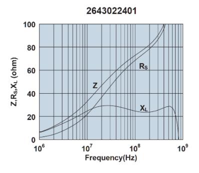
Impedance, reactance, and resistance vs. frequency.
