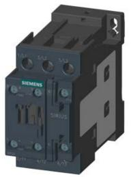
CONTACTOR, AC-3, 5.5KW/400V, 1NO+1NC, DC 60V, 3-POLE, SZ S0 SCREW TERMINAL
