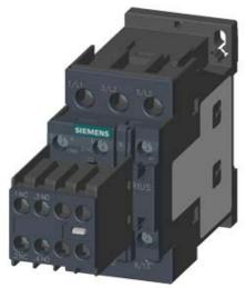
CONTACTOR, AC-3, 7.5KW/400V, 2NO+2NC, AC 110V 50HZ 120V 60HZ, 3-POLE, SZ S0 SCREW TERMINAL REMOVABLE AUX. SWITCH
