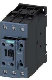
RAIL-CONTACTOR, AC-3, 30KW/400V, 1NO+1NC, 24VDC, 0.7...1.25\*US, WITH VARISTOR, 3-POLE, SIZE S2, SCREW TERMINAL
