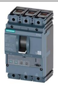
CIRCUIT BREAKER 3VA2 IEC FRAME 100 BREAKING CAPACITY CLASS M ICU=55KA @ 415 V 3POLE, LINE PROTECTION ETU330, LIG, IN=25A OVERLOAD PROTECTION IR=10A ...25A SHORT CIRCUIT PROTECTION II=1,5...12 X IN GROUNDFAULTPROTECTION IG=0,2... 1 X IN, TG=0,1/0,3MS CABLE CONNECTION
