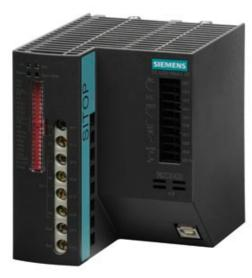
SITOP DC UPS MODULE 40A WITHOUT INTERF. SITOP DC USV MODULE 24 V/40 A UNINTERRUPTIBLE POWER SUPPLY WITHOUT INTERFACE INPUT: 24 V DC/43 A OUTPUT: 24 V DC/40 A
