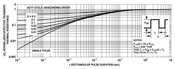
Figure 12. Transient Thermal Response Curve
