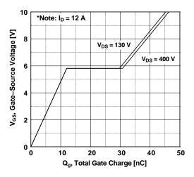
Figure 6. Gate Charge Characteristics
