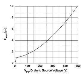
Figure 11. E<sub>OSS</sub> vs. Drain to Source Voltage
