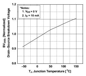
Figure 7. Breakdown Voltage Variation vs. Temperature
