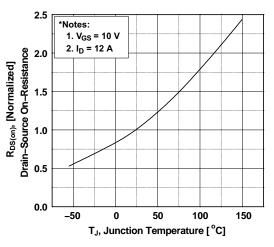
Figure 8. On-Resistance Variant vs. Temperature
