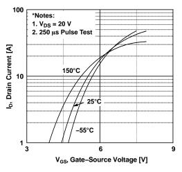
**Figure 2. Transfer Characteristics**
