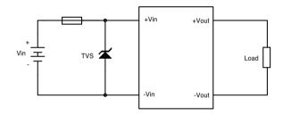
The QSB300 series converters have no internal fuse. In order to achieve maximum safety and system protection, always use an input line fuse. We recommended a 60A time delay fuse for 24Vin models, and 30A for 48Vin models. It is recommended that the circuit have a transient voltage suppressor diode TVS (24 Vin SMCJ40A: 48 Vin, SMCJ78A) across the input terminal to protect the unit against surge or spike voltage and input reverse voltage (as shown).
