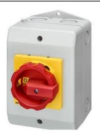
MAIN/EMERG. STOP SWITCH 4-POLE IU=63, P/AC-23A AT 400V=22KW 1 N-TERMINAL INSULATION-ENCLOSED, IP65 ROTARY ACTUATOR RED/YELLOW (EMERG. STOP) METRIC SCREW CONNECTION
