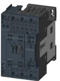
4NO CONTACTOR, AC1: 35A AC 230V 50HZ 4-POLE, 4NO, SZ: S0, SPRING-LOADED TERMINAL 1NO+1NC INTEGR.
