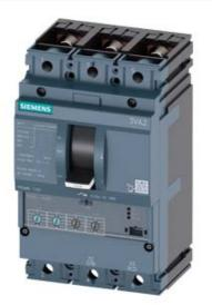
CIRCUIT BREAKER 3VA2 IEC FRAME 100 BREAKING CAPACITY CLASS M ICU=55KA @ 415 V 3POLE, LINE PROTECTION ETU350, LSI, IN=63A OVERLOAD PROTECTION IR=25A ...63A SHORT CIRCUIT PROTECTION ISD=1,5... 10 X IR, II=12 X IN BUSBAR CONNECTION
