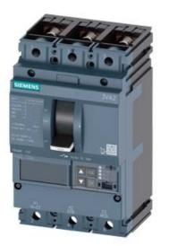
CIRCUIT BREAKER 3VA2 IEC FRAME 100 BREAKING CAPACITY CLASS M ICU=55KA @ 415 V 3POLE, LINE PROTECTION ETU560, LSIG, IN=63A OVERLOAD PROTECTION IR=25A ...63A SHORT CIRCUIT PROTECTION ISD=0,6..10X IN, II=1,5..12X IN NEUTRAL PROTECTION OPTIONAL WITH EXT. CT,UPTO 160% GROUNDFAULT, SWITCHABLE IG=0,2... 1 X IN, TG=0,050,8MS BUSBAR CONNECTION
