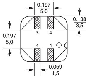
\* For optional tin-lead and tin-silver-copper terminations, dimensions are for the mounted part. Dimensions before mounting can be an additional 0.012 inch (0,3 mm).
