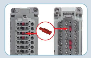
Each position of the coding pin used on the female insert must correspond to an unused position on the male insert.
