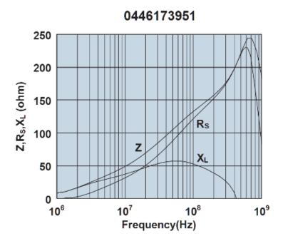
Impedance, reactance, and resistance vs. frequency.
