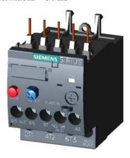
OVERLOAD RELAY 0.70...1.0 A FOR MOTOR PROTECTION SZ S00, CLASS 10, F. MOUNTING ONTO CONTACTOR MAIN CIRCUIT: SCREW TERMINAL AUX. CIRCUIT: SCREW TERMINAL MANUAL-AUTOMATIC-RESET
