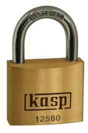
~ Hardened steel shackle ~ Double bolted locking mechanism ~ Solid brass body ~ Anti pick mushroom pins ~ Paracentric keyway ~ Supplied with 2 keys ~ Keyed alike, all padlocks of this order code can be opened with the same key ~ Padlock width: 60 mm ~ Shackle diameter: 9,5 mm ~ Internal shackle height: 34 mm
