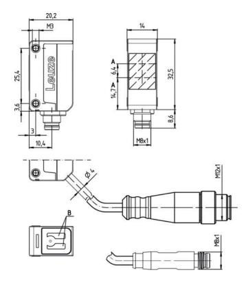
A Optical axis B Indicator diode
