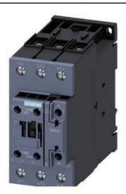
CONTACTOR,AC3:18.5KW/400V, 1NO+1NC, 24V AC 50HZ, 3-POLE, SIZE S2, SCREW TERMINAL UPRIGHT MOUNTING POSITION
