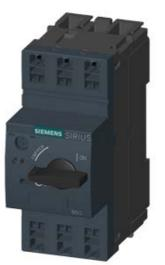
CIRCUIT-BREAKER SZ S00, FOR MOTOR PROTECTION, CLASS 10, A-RELEASE 7...10A, N-RELEASE 130A, SPRING-L. CONNECTION, STANDARD SW. CAPACITY
