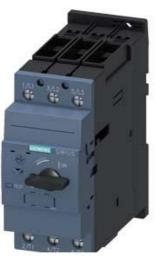
CIRCUIT BREAKER SIZE S2, FOR MOTOR PROTECTION, CLASS 10, A-RELEASE 14...20A, N-RELEASE 260A, SCREW TERMINAL, STANDARD BREAKING CAPACITY
