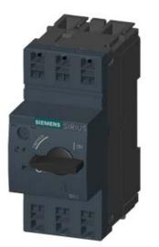
CIRCUIT-BREAKER SZ S00, FOR TRANSFORMER PROT. A-RELEASE1.1...1.6 A, N-RELEASE 33A SPRING-L. CONNECTION, STANDARD SW. CAPACITY
