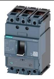
CIRCUIT BREAKER 3VA1 IEC FRAME 160 BREAKING CAPACITY CLASS M ICU=55KA @ 415 V 3-POLE, LINE PROTECTION TM240, ATAM, IN=125A OVERLOAD PROTECTION IR=87,5A ...125A SHORT CIRCUIT PROTECTION II=5...10 X IN BUSBAR CONNECTION
