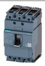
CIRCUIT BREAKER 3VA1 IEC FRAME 160 BREAKING CAPACITY CLASS N ICU=25KA @ 415 V 3-POLE, LINE PROTECTION TM210, FTFM, IN=32A OVERLOAD PROTECTION IR=32A FIXED SHORT CIRCUIT PROTECTION II=10 X IN CABLE CONNECTION
