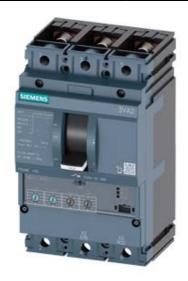
CIRCUIT BREAKER 3VA2 IEC FRAME 160 BREAKING CAPACITY CLASS C ICU=110KA @ 415 V 3POLE, LINE PROTECTION ETU350, LSI, IN=40A OVERLOAD PROTECTION IR=16A ...40A SHORT CIRCUIT PROTECTION ISD=1,5... 10 X IR, II=12 X IN BUSBAR CONNECTION
