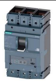
CIRCUIT BREAKER 3VA2 IEC FRAME 630 BREAKING CAPACITY CLASS H ICU=85KA @ 415 V 3-POLE, LINE PROTECTION ETU350, LSI, IN=400A OVERLOAD PROTECTION IR=160A ...400A SHORT CIRCUIT PROTECTION ISD=1,5... 10 X IR, II=12 X IN BUSBAR CONNECTION
