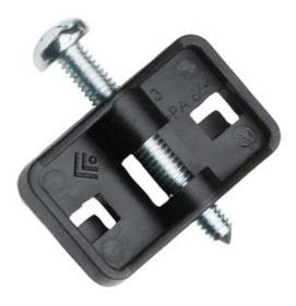
PLASTIC MOUNTING CLIPS FOR TD 17, OP 7, OP 17, OP 73, OP 77A/B, TP/OP 17X NOT FOR TP 177 4", PUSHBUTTONPANEL, KEYPANEL, DESIGN BLANK FRONT; KP300 BASIC MONO, BASIC PANELS 2ND GENERATION, KTP400 COMFORT, USB-HUB, SHEET THICKNESS 2 TO 6 MM AMOUNT: SEE TECHNICAL DATA
