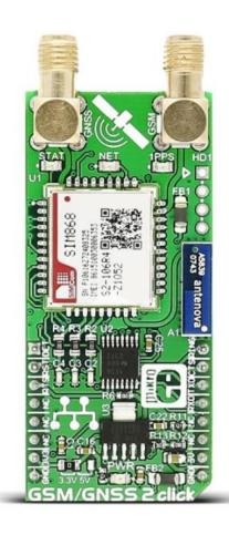
**GSM/GNSS 2** click combines GPS/GLONASS location tracking with GSM module capability for mobile communication.
