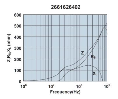
Impedance, reactance, and resistance vs. frequency.
