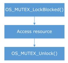
A mutex contains a counter that keeps track of how many times the mutex has been claimed by calling  $os_{tock}()$  or  $os_{tock}()$  or  $os_{tock}()$  by a particular task. It is released when that counter reaches zero, which means the  $os_{tock}()$  routine must be called exactly the same number of times as  $os_{tock}()$  or  $os_{tock}()$  or  $os_{tock}()$ . If it is not, the mutex remains blocked for other tasks.
