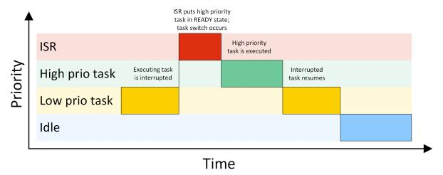
Preemptive multitasking may be switched off in sections of a program where task switches are prohibited, known as critical regions. embOS itself will also temporarily disable preemptive task switches during critical operations, which might be performed during the execution of some embOS API functions.
