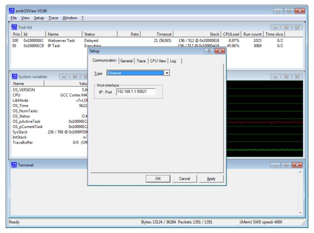
In the Communication tab, choose "Ethernet" in the Type selection list box. In the Host interface box, configure the IP address of your target and the port number 50021.
