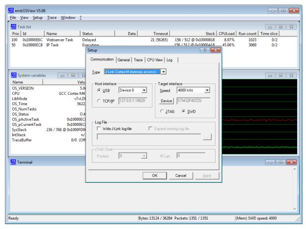
In the Communication tab, choose "J-Link Cortex-M (memory access)", "J-Link RX (memory access)" or "J-Link ARM7/9/11 (DCC)" in the  ${\tt Type}$  selection list box.
