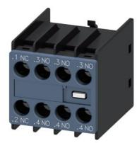
Auxiliary switch Front side, 3 NO + 1 NC Current path 1 NC, 1 NO, 1 NO, 1 NO For 3RH2 and 3RT2 Screw terminal .1/.2, .3/.4, .3/.4, .3/.4
