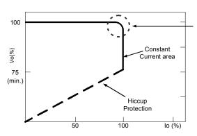
Typical LED power supply I-V curve
