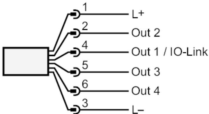
OUT1: switching output IO-Link
