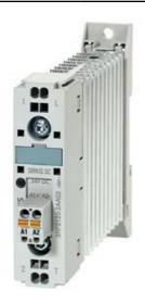
SEMI-COND. CONTACTOR 3RF2,1-PH. AC 51 20 A 40 DEGREES C 48-460 V / 24 V DC SHORT-CIRC. RESIST. WITH SPRING-LOADED CONNECTION
