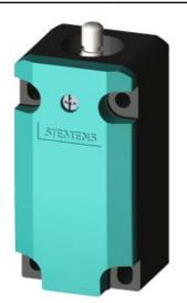
BASIC SWITCH FOR POSITION SWITCH 3SE513, PLASTIC ENCLOSURE, TO EN50041 1X(M20X1.5) 1NO/1NC QUICK-ACTION CONTACTS W/O ACTUATOR HEAD
