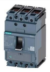
CIRCUIT BREAKER 3VA1 IEC FRAME 160 BREAKING CAPACITY CLASS M ICU=55KA @ 415 V 3-POLE, LINE PROTECTION TM220, ATFM, IN=50A OVERLOAD PROTECTION IR=35A ...50A SHORT CIRCUIT PROTECTION II=10 X IN CABLE CONNECTION
