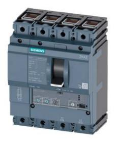
CIRCUIT BREAKER 3VA2 IEC FRAME 160 BREAKING CAPACITY CLASS C ICU=110KA @ 415 V 4POLE, LINE PROTECTION ETU320, LI, IN=40A OVERLOAD PROTECTION IR=16A ...40A SHORT CIRCUIT PROTECTION II=12 X IN NEUTRAL PROTECTION ADJUSTABLE(OFF,100%) CABLE CONNECTION
