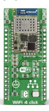
**WiFi 4 click** carries <u>SPWF01SA</u>, a complete standalone WiFi module with a single-chip 802.11 b/g/n transceiver, a 32-bit STM32 MCU, along with a built-in 2.4 GHz ISM band antenna.
