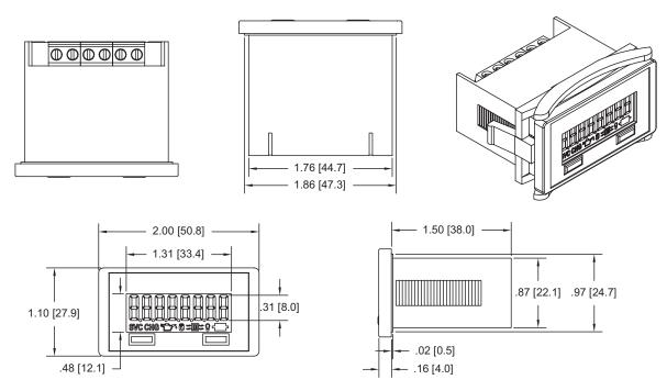
Panel Cutout: 1.79" [45.5mm] x 0.89" [22.6mm] Recommended Panel Thickness: 0.875" [22.2mm]
