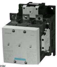
VAC. CONTACTOR, 110KW/400V/AC-3 AC(40...60HZ)/DC OPERATION UC 96-127V AUXILIARY CONTACTS 2NO+2NC 3-POLE, SIZE S10 BAR CONNECTIONS ELECTRONIC OPERATING MECHANISM WITH 24V DC PLC INTERFACE
