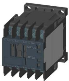
CONTACTOR, AC-3, 5.5KW/400V, 1NC, AC110V 50HZ, 120V 60HZ 3-POLE, SZ S00 RING CABLE LUG CONNECTION
