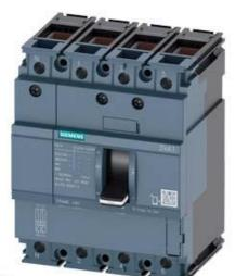
CIRCUIT BREAKER 3VA1 IEC FRAME 160 BREAKING CAPACITY CLASS N ICU=25KA @ 415 V 4-POLE, LINE PROTECTION TM210, FTFM, IN=100A OVERLOAD PROTECTION IR=100A FIXED SHORT CIRCUIT PROTECTION II=10 X IN NEUTRAL PROTECTION 100% CABLE CONNECTION
