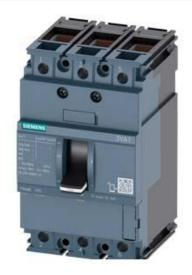
CIRCUIT BREAKER 3VA1 IEC FRAME 160 BREAKING CAPACITY CLASS H ICU=70KA @ 415 V 3-POLE, LINE PROTECTION TM210, FTFM, IN=20A OVERLOAD PROTECTION IR=20A FIXED SHORT CIRCUIT PROTECTION II=10 X IN CABLE CONNECTION
