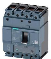
CIRCUIT BREAKER 3VA1 IEC FRAME 160 BREAKING CAPACITY CLASS H ICU=70KA @ 415 V 4-POLE, LINE PROTECTION TM240, ATAM, IN=63A OVERLOAD PROTECTION IR=44,1A ...63A SHORT CIRCUIT PROTECTION II=5...10 X IN NEUTRAL UNPROTECTED CABLE CONNECTION
