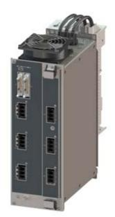
SIPLUS HCS4300 POM4320 BUSBAR MOUNTING (IEC). POWER OUTPUT MODULE FOR MOUNTING ON POWER RAIL SYSTEM. REDESIGN WITH INCREASED EMC RESISTANCE. WITH 9 POWER OUTPUTS EACH MAX. 7680 W (WITH CONTROL MODE HALF-WAVE CONTROL: DEPENDING ON THE INRUSH CURRENT OF THE ELECTRIC LOAD THERE IS A LIMITATION OF MAX. 4000 W)
